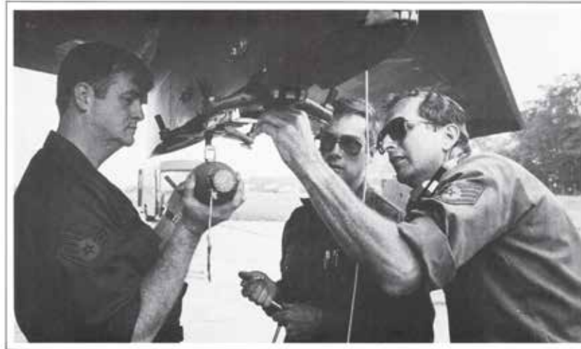
(left to right) Staff Sergeants Robert M. McArdle, Ronald E. Snyder and Terrance A. Buechel, 112th Tactical Fighter Group, Pennsylvania Air National Guard, load a 25-pound practice bomb on an A-7D
